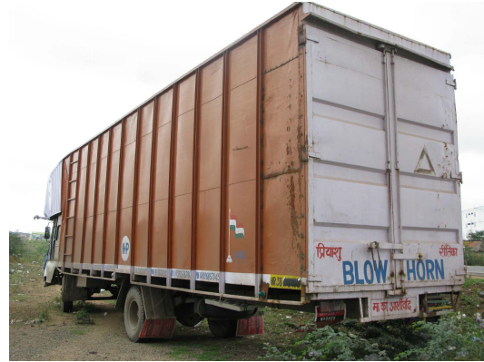
Figure 5: Heavy Truck Without Functioning Brake Lights, Rear Reflectors or Underride Protection During the 2010 Coimbatore Study
